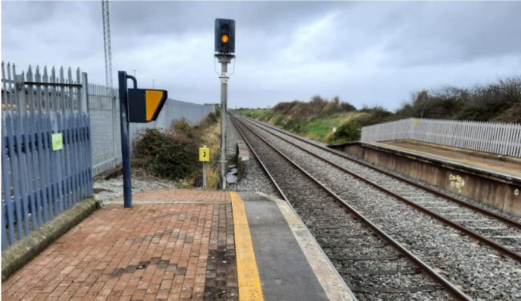
**Figure 5-22: Signal mast at the north end of the station**
